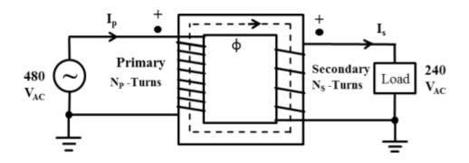
(a) As discussed in this segment, when voltage must be reduced to accommodate the load, the transformer must be connected in a step down configuration. Therefore, the answer is: **step down configuration**.
