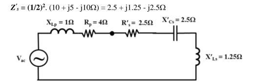
Then, combination of the primary impedance and the total reflected secondary impedance would result in the equivalent impedance  $Z_{eq}$ :
